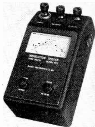
A commercial meter, the Dawe Instruments Type 402B Insulation Tester, which operates on the grid-current principle.
